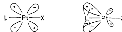
Figure 8. The rotation necessary to remove steric interference in a trans -disubstituted olefin complex.
